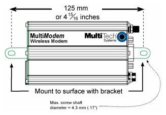
Drill the mounting holes at the desired mounting location (if applicable).
