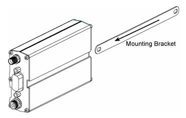
4. Attach the modem with two screws to the mounting surface at the desired location on the equipment.
